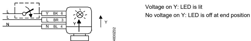
The LED is lit when the actuator stem protrudes, retracts, or the valve fully opens. The LED goes out when the actuator stem protrudes to the valve's fully closed position.
